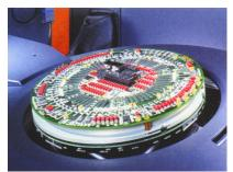
Many integrated circuits used in high stress environments (for example, automobile under-hood) must be qualified at high temperatures to ensure they meet their design specifications. Automated Test Equipment (ATE)
