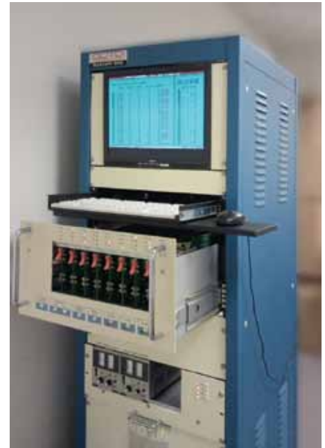
Fig 2. Coto Technology System 300 Relay Life Test System
