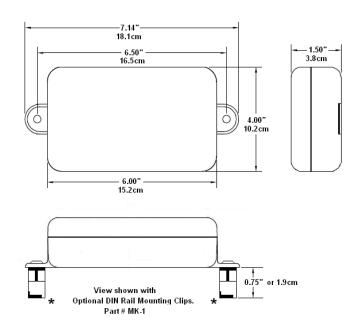
The D8000 series modules can be easily adapted to a DIN rail using the DGH MK-1 mounting kit shown in view above.
