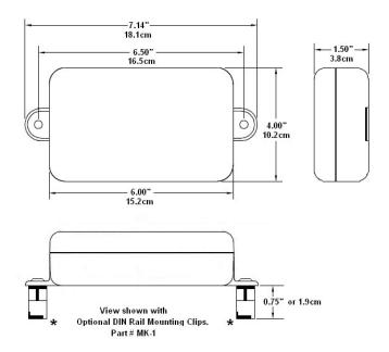
The D7000 series modules can be easily adapted to a DIN rail using the DGH MK-1 mounting kit shown in view above.
