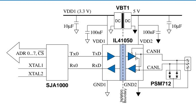
This bulletin describes a complete isolated CAN node including a dc-dc convertor and additional bus transient voltage protection.
